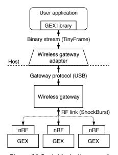
**Figure 11.2:** A block diagram of the wireless connection
