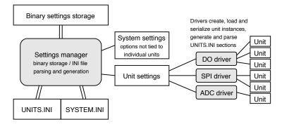
Figure 9.2: Structure of the settings subsystem
