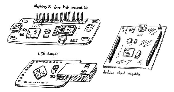
**Figure 2.2:** A sketch of three possible form factors for the GEX hardware prototype. Note the ESP8266 module which was considered as an option for wireless access but was eventually not used due to it's high current usage, unsuitable for battery operation.
