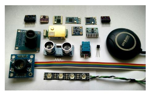
**Figure 1.1:** A collection of intelligent sensors and devices, most on breadboard adapters: (from top left) a waveform generator, a gesture detector, a LoRa and two Bluetooth modules, an air quality and pressure sensor, a  $CO_2$  sensor, a digital compass, an accelerometer, a GPS module, a camera, an ultrasonic range finder, a humidity sensor, a 1-Wire thermometer, a color detector and an RGB LED strip.
