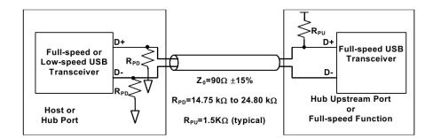
**Figure 4.5:** Pull-up and pull-down resistors of a Full Speed function, as prescribed by the USB specification rev. 2.0
