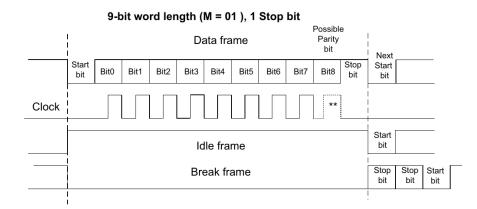
**Figure 7.1:** UART frame, as shown by the STM32F072 Reference Manual. Break frames are used by some UART based protocols, like LIN (Local Interconnect Network).
