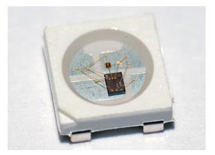
Figure 7.6: A close-up photo of the WS2812B package, showing the LED driver IC
