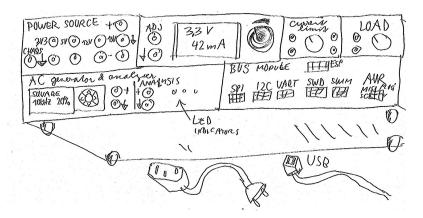
**Figure 1.2:** An early (2016) sketch of a universal bench device including a power supply, electronic load, a signal generator and a bus module. The bottom half of the panel is in a large part implemented by GEX.
