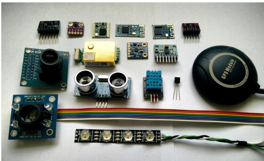
**Figure 1.1:** A collection of intelligent sensors and devices, most on breadboard adapters: (from top left) a waveform generator, a gesture detector, a LoRa and two Bluetooth modules, an air quality and pressure sensor, a CO<sub>2</sub> sensor, a digital compass, an accelerometer, a GPS module, a camera, an ultrasonic range finder, a humidity sensor, a 1-Wire thermometer, a color detector and an RGB LED strip.
