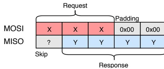
Figure 12.2: SPI transaction using the QUERY command
