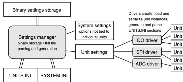
**Figure 9.2:** Structure of the settings subsystem
